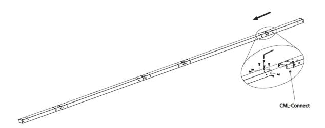
5. Slide completed vertical into CML- CARH and center.
