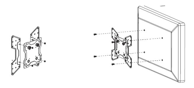
9. Hook TVs onto CM-CARTV and secure into place with washers and screws (Level TVs before tightening screws fully). Slide monitors together to eliminate gaps between TVs and then tighten brackets from step 7 fully to secure into place.
