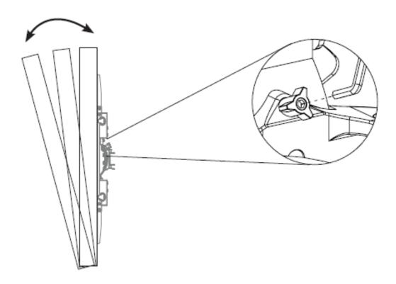
11. Each CM-CARTV has independent vertical micro-adjustments. If necessary, align TVs vertically using supplied wrench to raise or lower.
