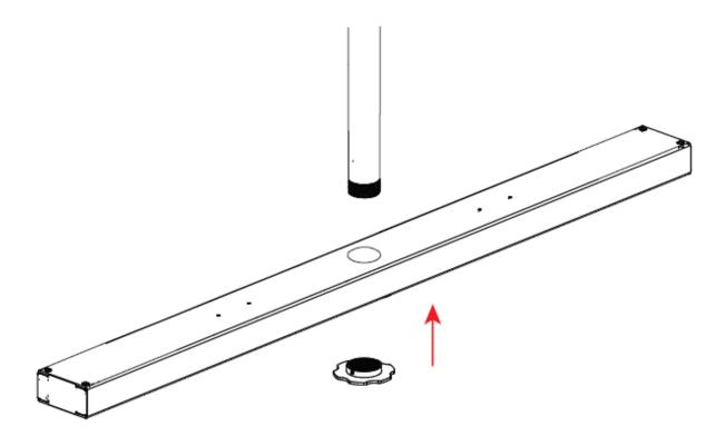
Tighten retaining collar by making several turns and lock into place using two security set screws.
