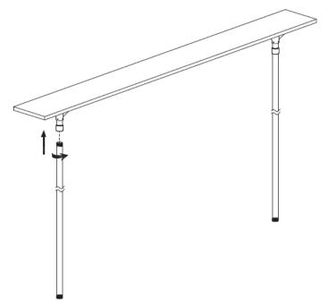
3. Attach CML-CARH to pipes and secure with pre-installed set screws.
