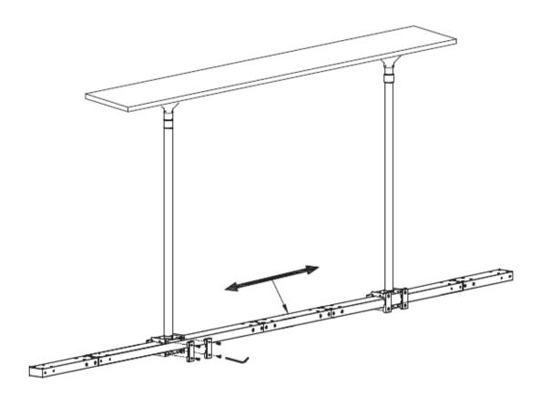
7. Attach CM-CARTV to vertical with brackets and screws. Do not tighten fully. This will allow adjustment vertically for different TV sizes.
