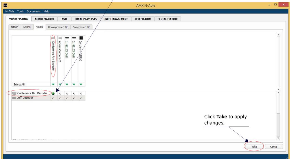
**FIG. 18** Seamless Switching Using the Video Matrix
