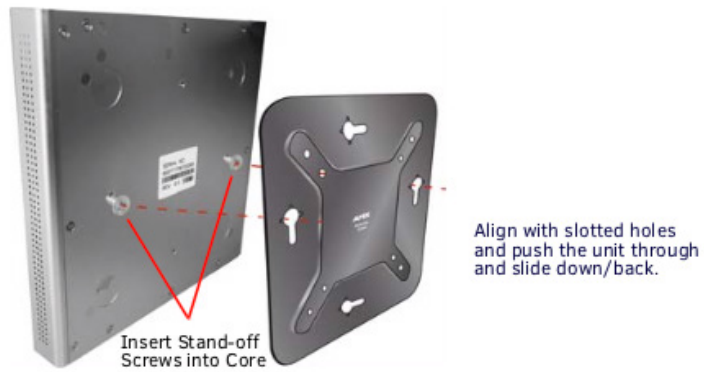
FIG. 15 ATTACH STAND-OFF SCREWS, INSERT THROUGH BACKPLATE
