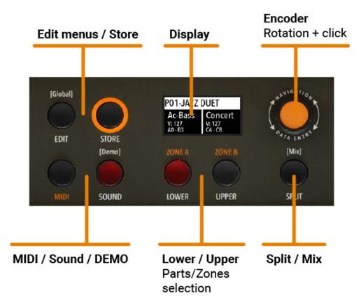
The main HOME display of the Numa Compact is the one shown at power on and it's divided in 3 main areas: the top area shows the current Program number and name, the left and right lower areas are related to the Lower and Upper Sound sections, in SOUND mode, and to the Zone A and Zone B sections, in MIDI Mode.
