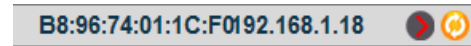
Figure 5: rotary' icon yellow color at right indicates firmware update for this unit is available
